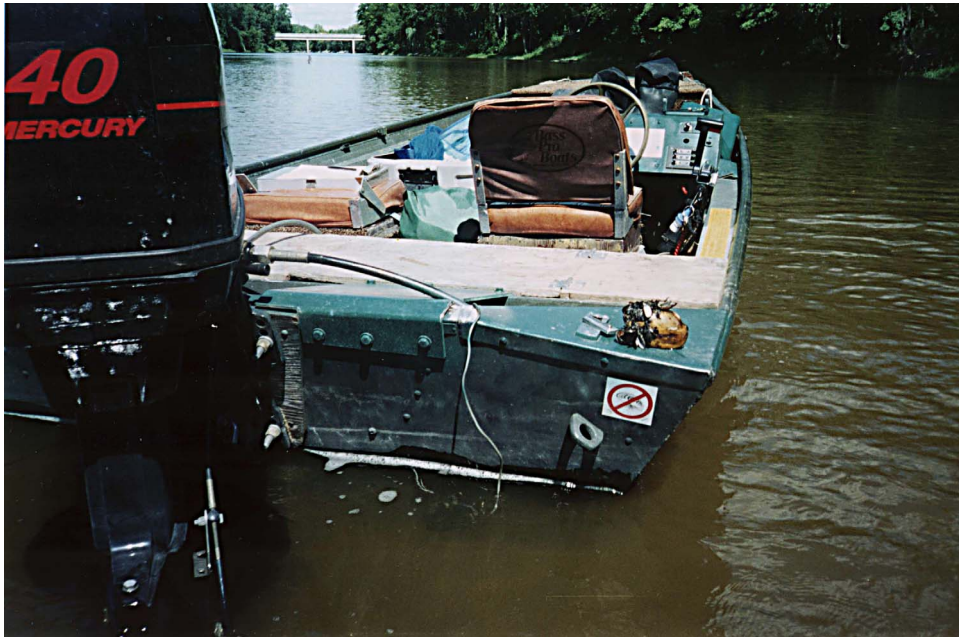
Figure 1. Boat with jet drive outboard engine used during surveys. Photo by Pete Badra.
